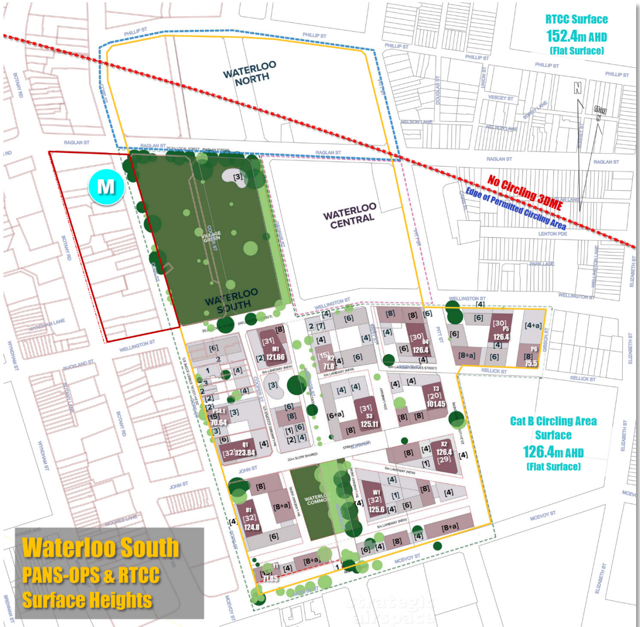
Figure 9 — PANS-OPS & RTCC/MVA Height Constraints across the Waterloo Precinct
